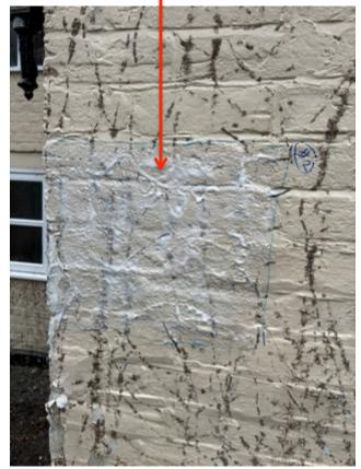
• All test panels subjected to super heated water at 150°C and at 40 bar pressure using the DOFF<sup>TM</sup> system to remove modern masonry paint:
