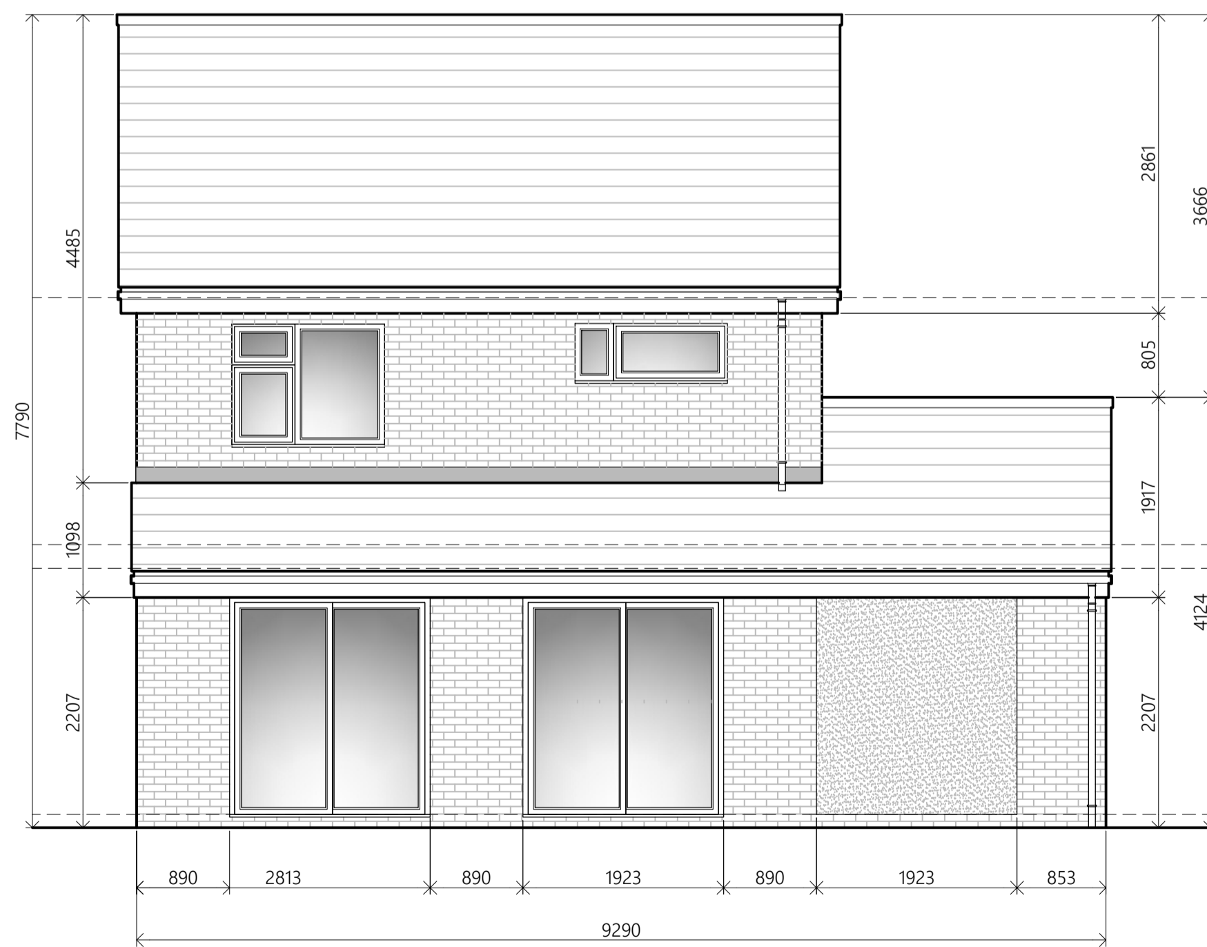
PROPOSED REAR ELEVATION SCALE 1:50
