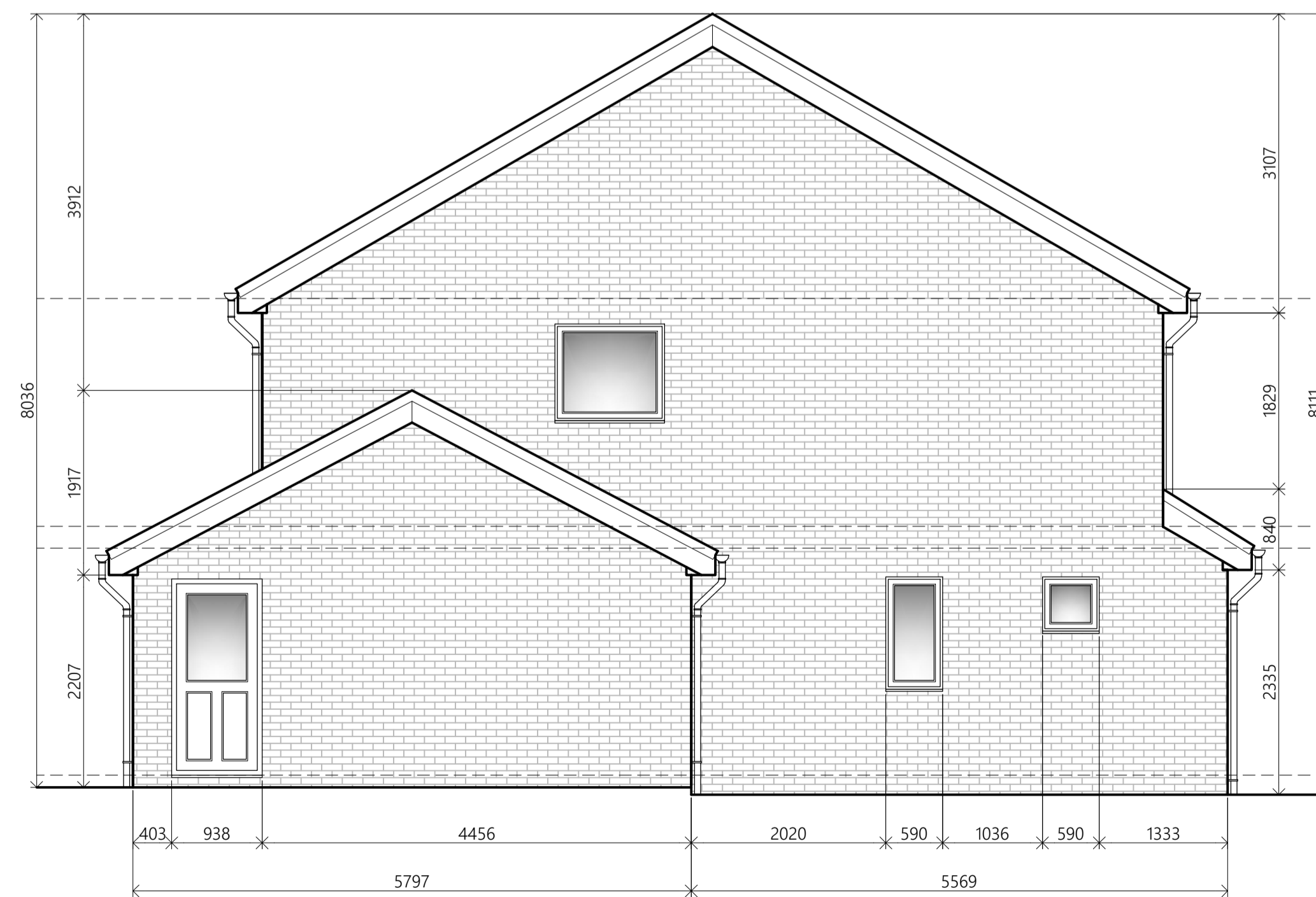
PROPOSED SIDE ELEVATION SCALE 1:50
