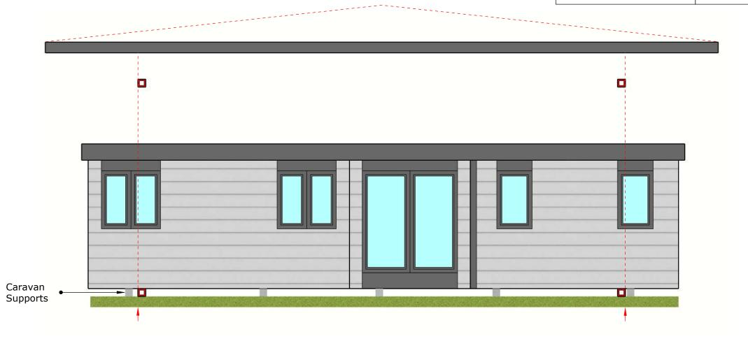
Roof Covering: EPDM seamless roof covering with 10mm gravel top coat.
