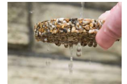
Resin bound gravel to front of house (parking areas)
