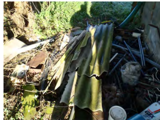
Photo 6: Broken asbestos cement board in Structure 3
