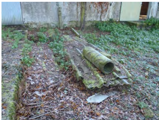
Photo 3: Made ground in front of Structure 4 including ACM
