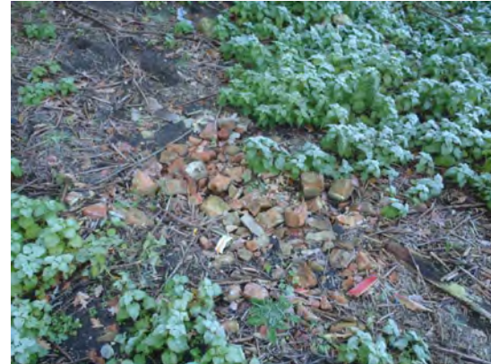
Photo 4: Asbestos cement board fragments on bare soil in front of Structure 4
