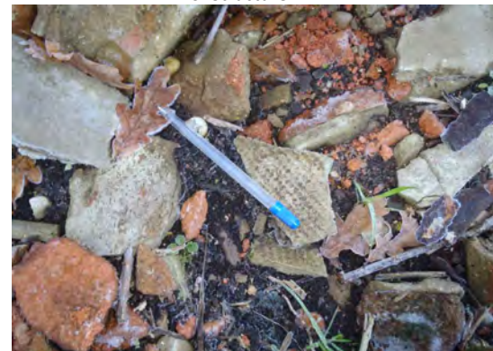
Photo 4: Asbestos cement board fragments on bare soil in front of Structure 4
