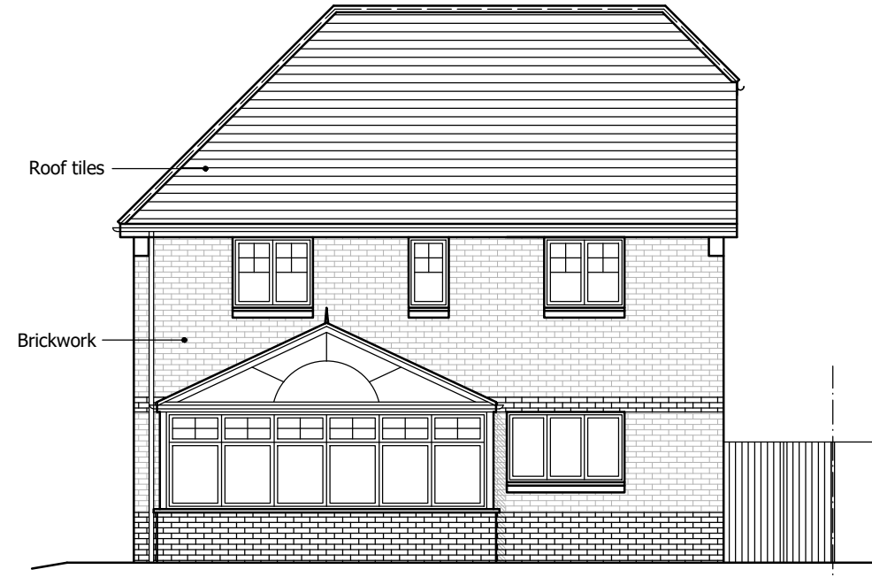
PROPOSED REAR ELEVATION scale 1:100
