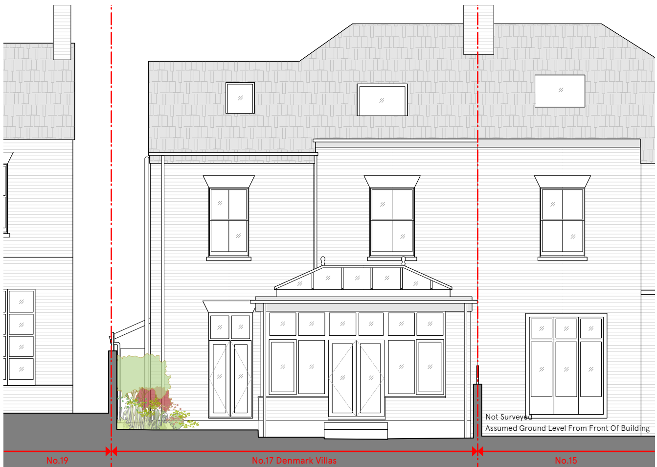
Above: Existing rear west elevation, scale 1:100.
