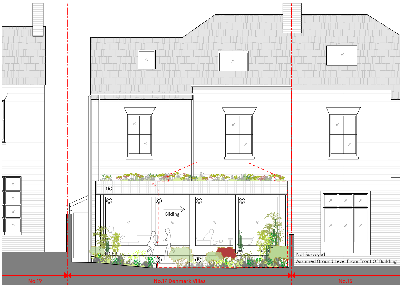
Above: Proposed rear west elevation, scale 1:100.
