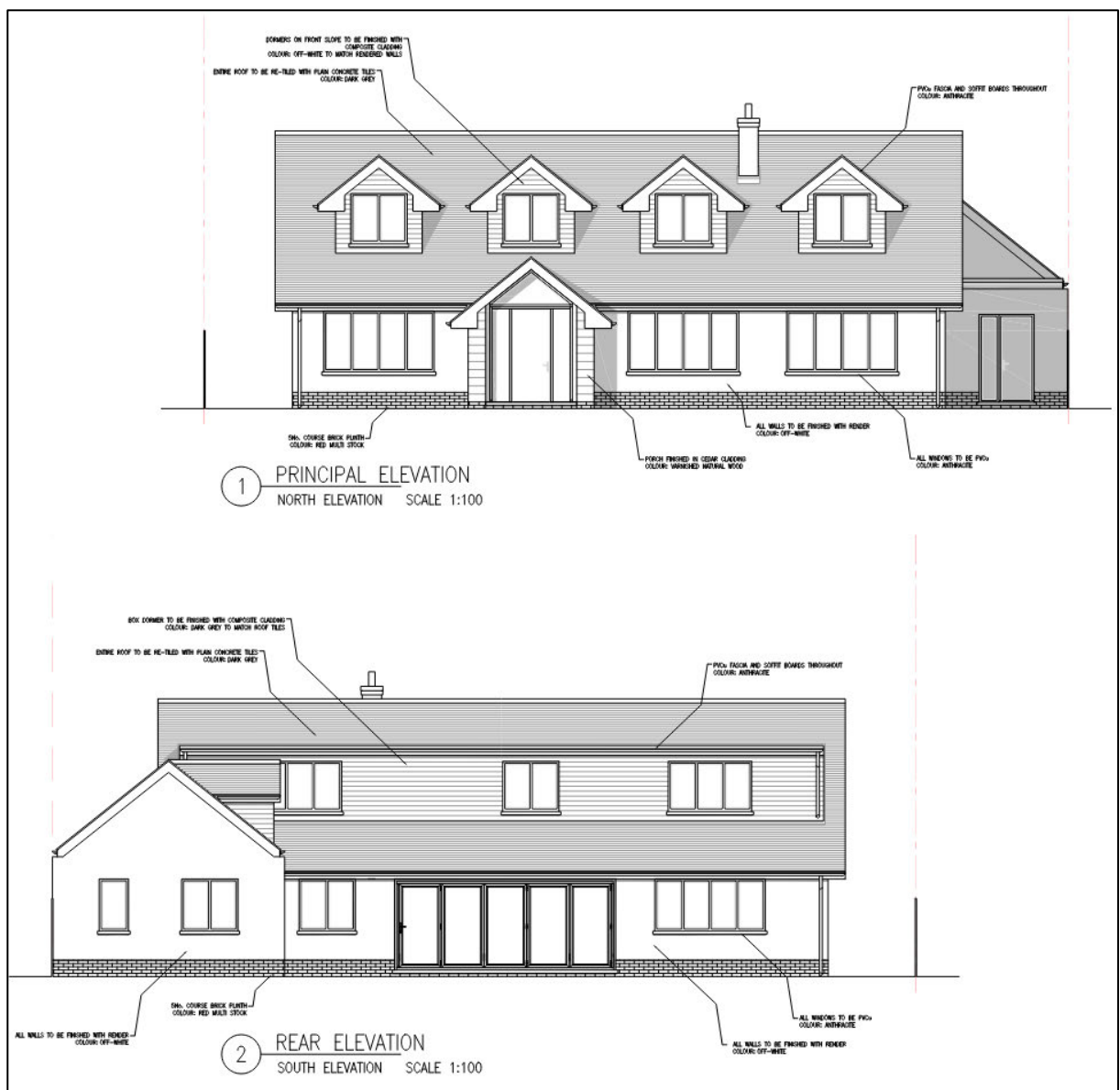
Figure 3: The approved front and rear elevations
