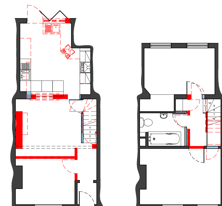
GF AND FF DEMOLITIONS PLAN SCALE: 1:100
