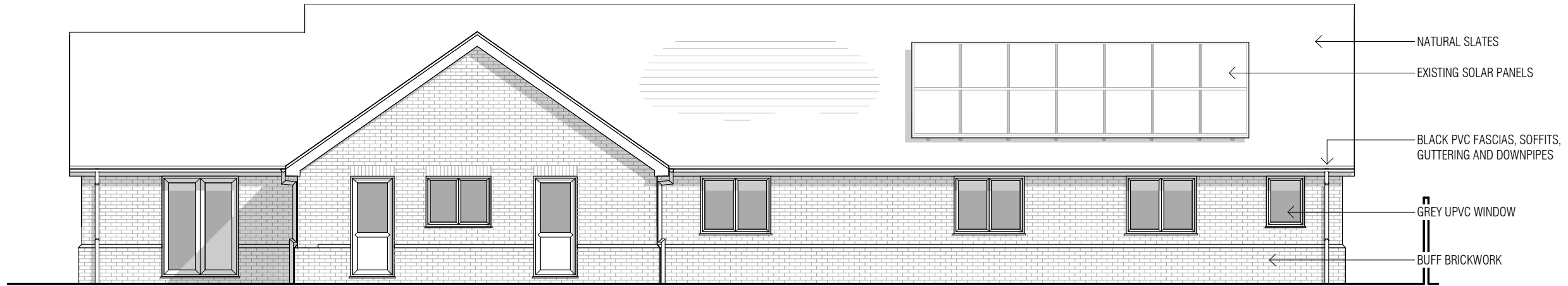
1 EXISTING EAST ELEVATION 1:100
