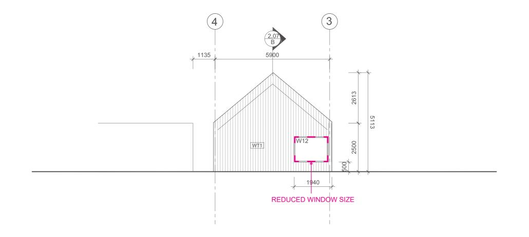
WT1 Timber cladding Vertical
