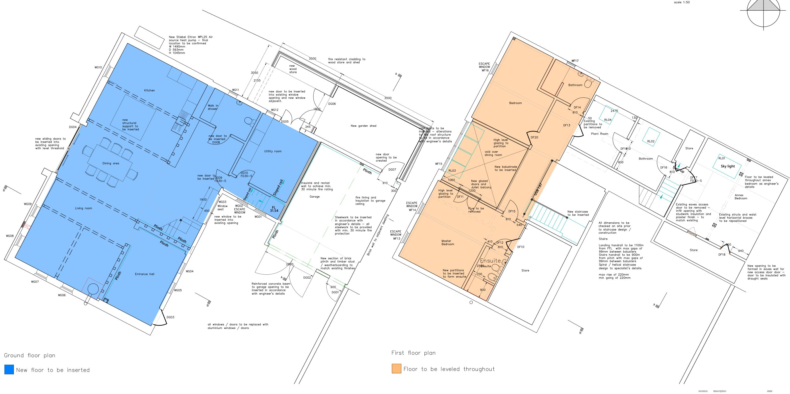
Floor — Ground Floor Upgrade to Existing  $(U-Value 0.23W/m^2K)$
