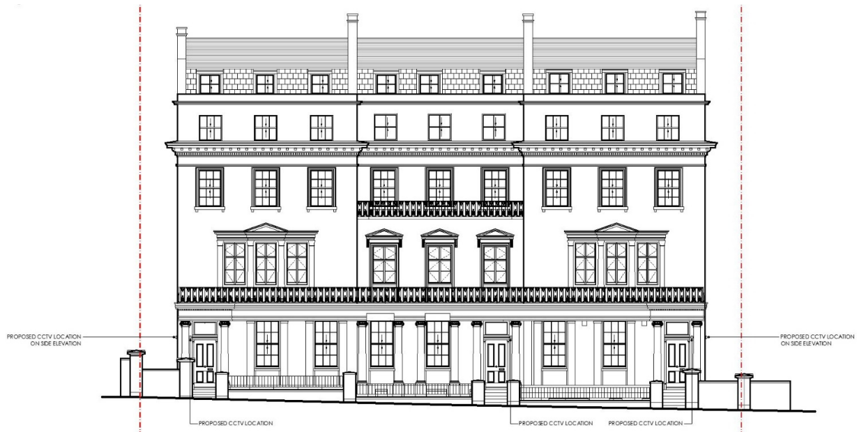
Above: Drawing showing the locations of the proposed cctv camera within the front elevation.
