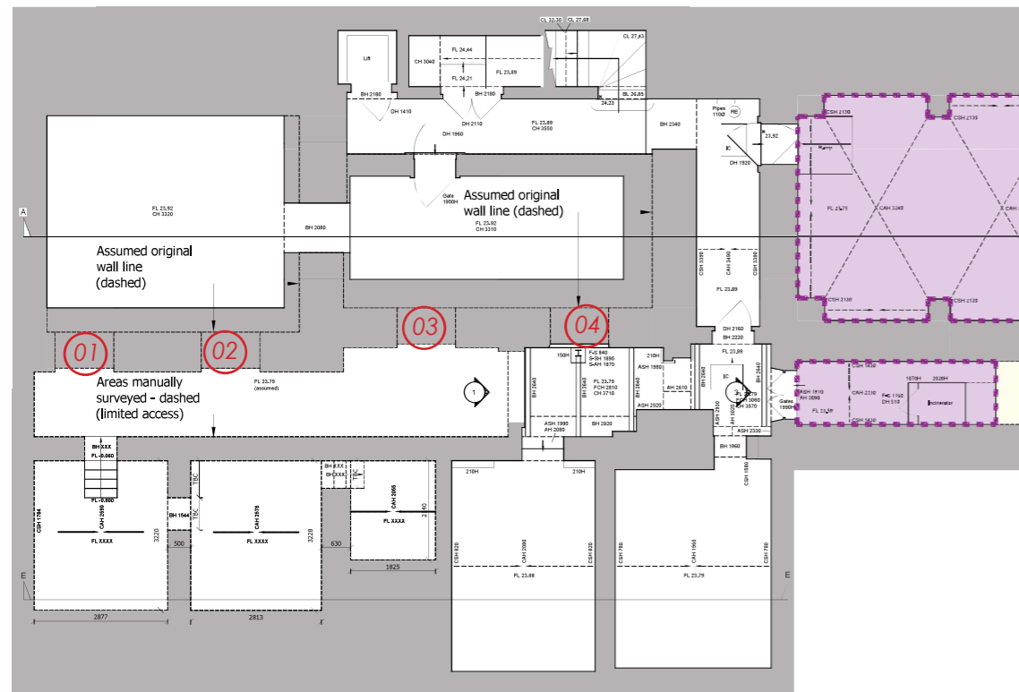
Part plan showing western lightwell and vaults
