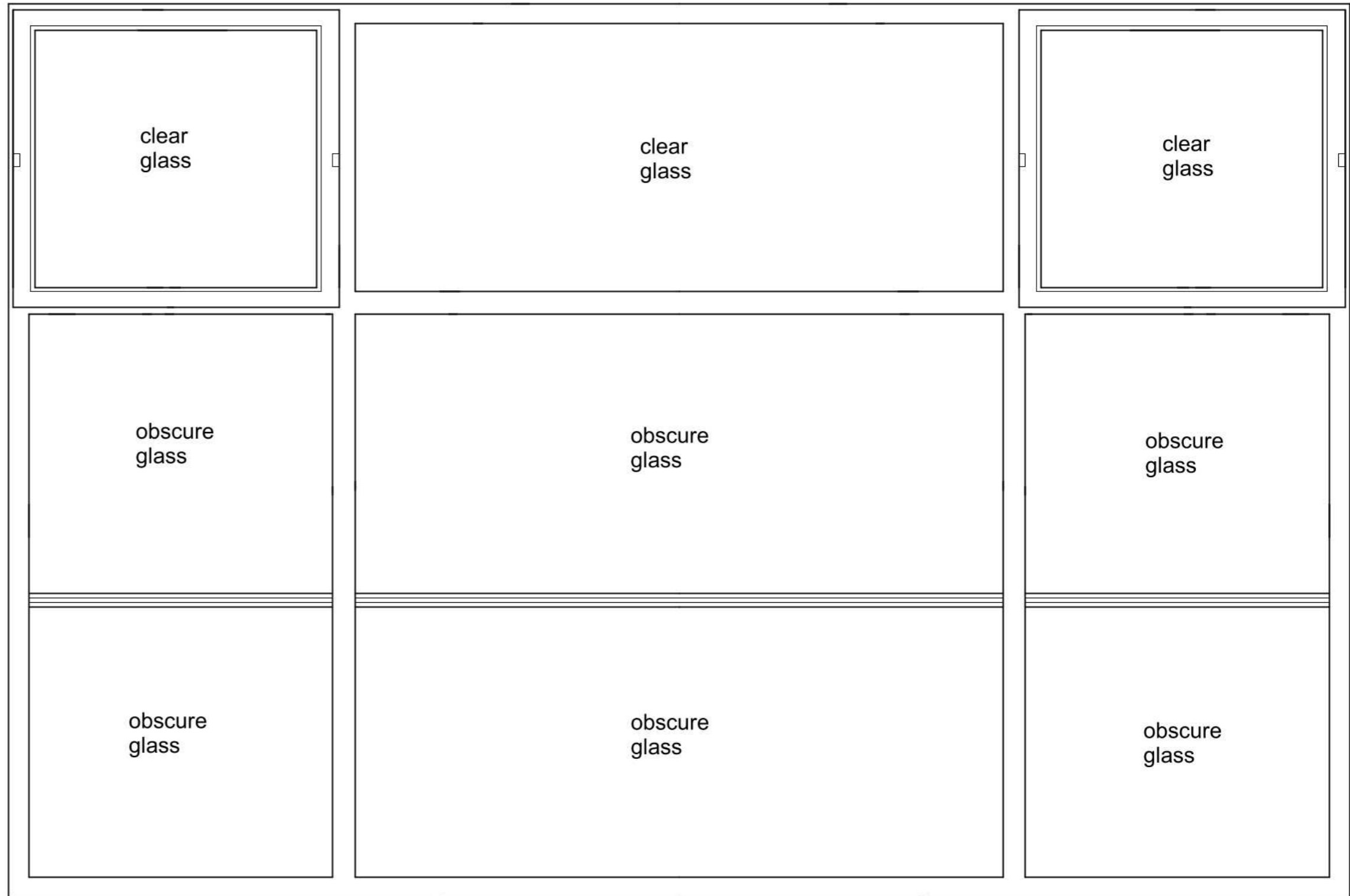
EXISTING METAL FRAME single glazed
