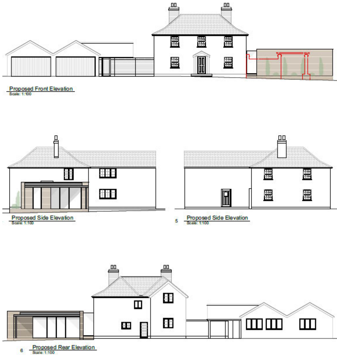
Figure 28 - Proposed elevations with the outline of the existing structure to be removed shown in red
