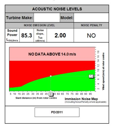
The noise map can be read by drawing a horizontal line from the recorded wind speed at hub (right hand side of the map) to where the red and green lines meet. Drawing a vertical line from
