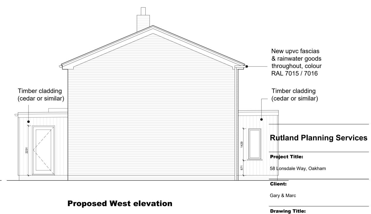
Proposed floor plan & elevations
