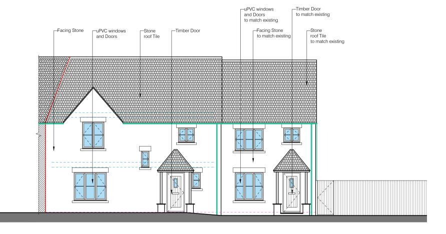
FRONT ELEVATION AS PROPOSED SCALE - 1:100@A1
