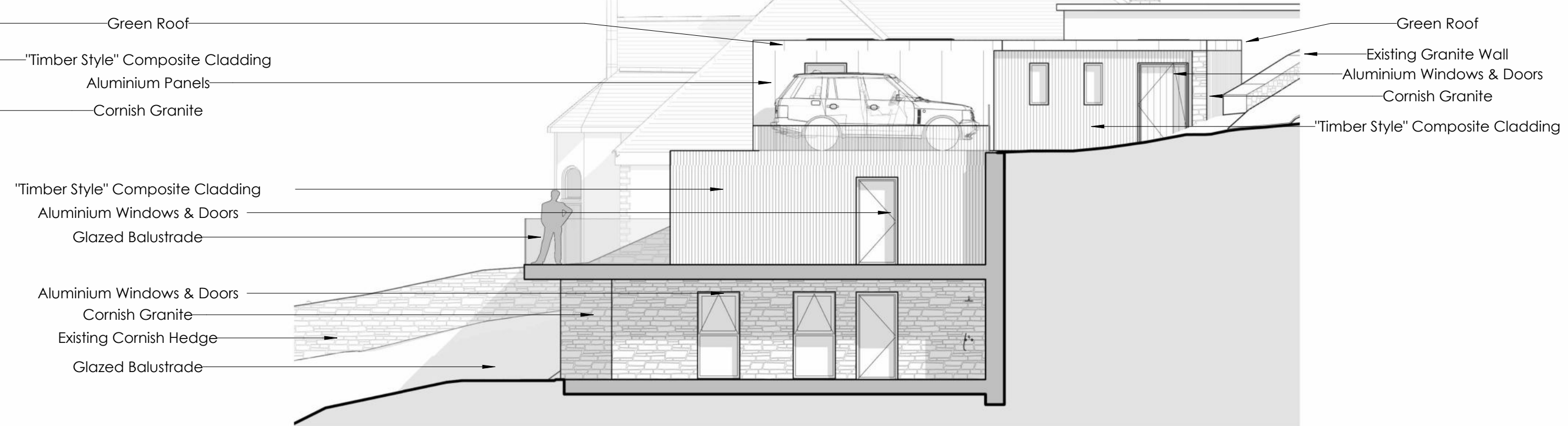
7 Proposed West Elevation 1 : 100
