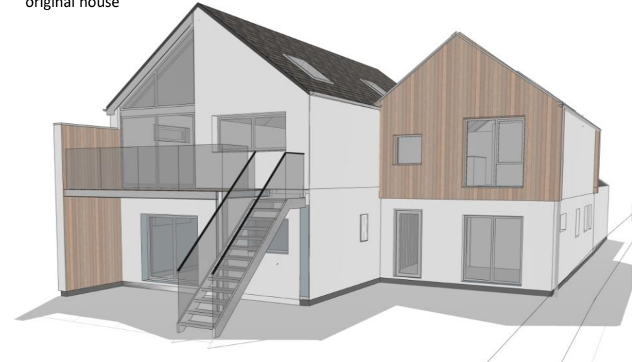
Image 4– Amended proposal with balcony roof cut back to the existing building line
