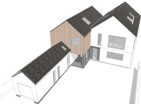
Image 2– Amended scheme with fibre cement slate roof. The image also shows the remodelling of the windows to the side of the garage
