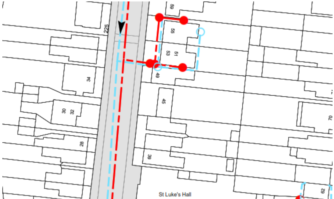
Figure 2: Thames Water Sewer record extract
