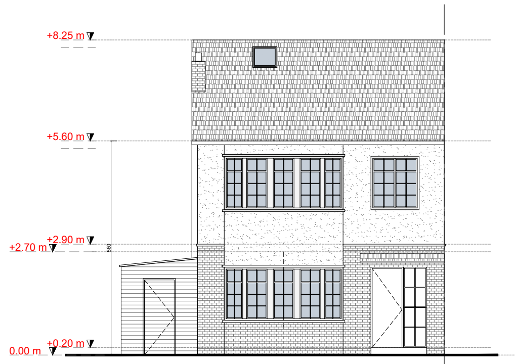
Existing Front Elevation
