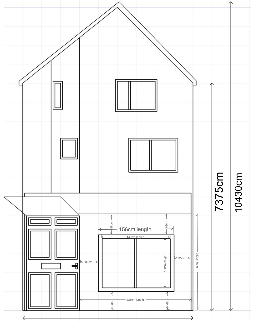
5250cm Proposed Front Elevation
