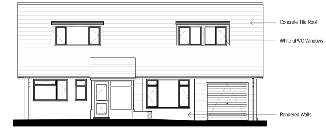
03 Front Elevation - Existing 1:100
