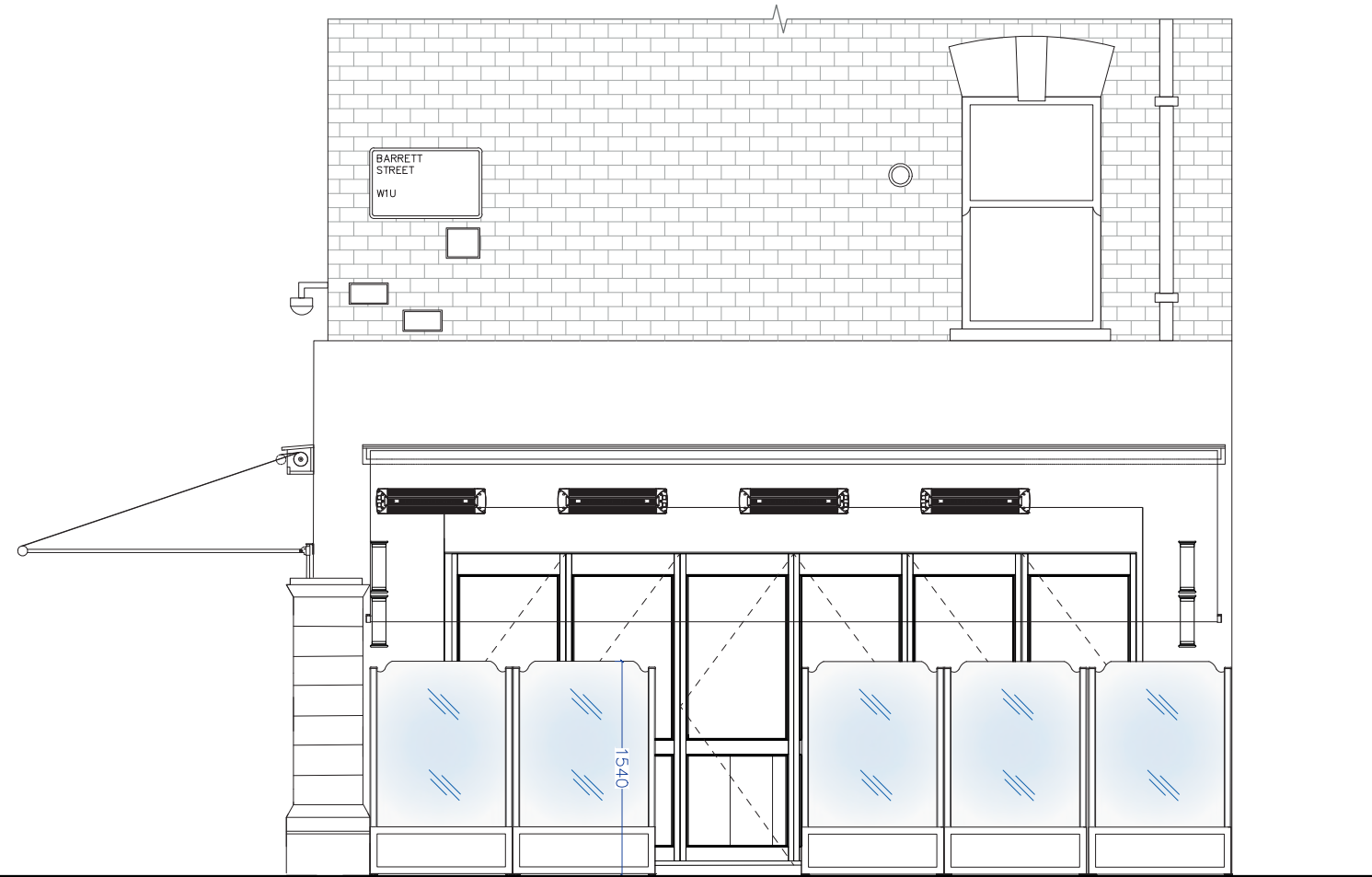
BARRETT STREET ELEVATION - SHOWING THE WINDBREAKERS
