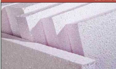
A compressible-fill material. It is used to prevent potential problems in foundations caused by moisture movement in soils, by being permanent shuttering for cast in-situ reinforced concrete, reducing pressure on ground beams in piled foundations and on the side of trench fill. \*For higher shrinkage or void values, consult the manufacturer.
