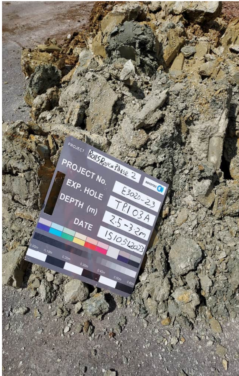
TP103A Spoil 2.50m to 3.20m
