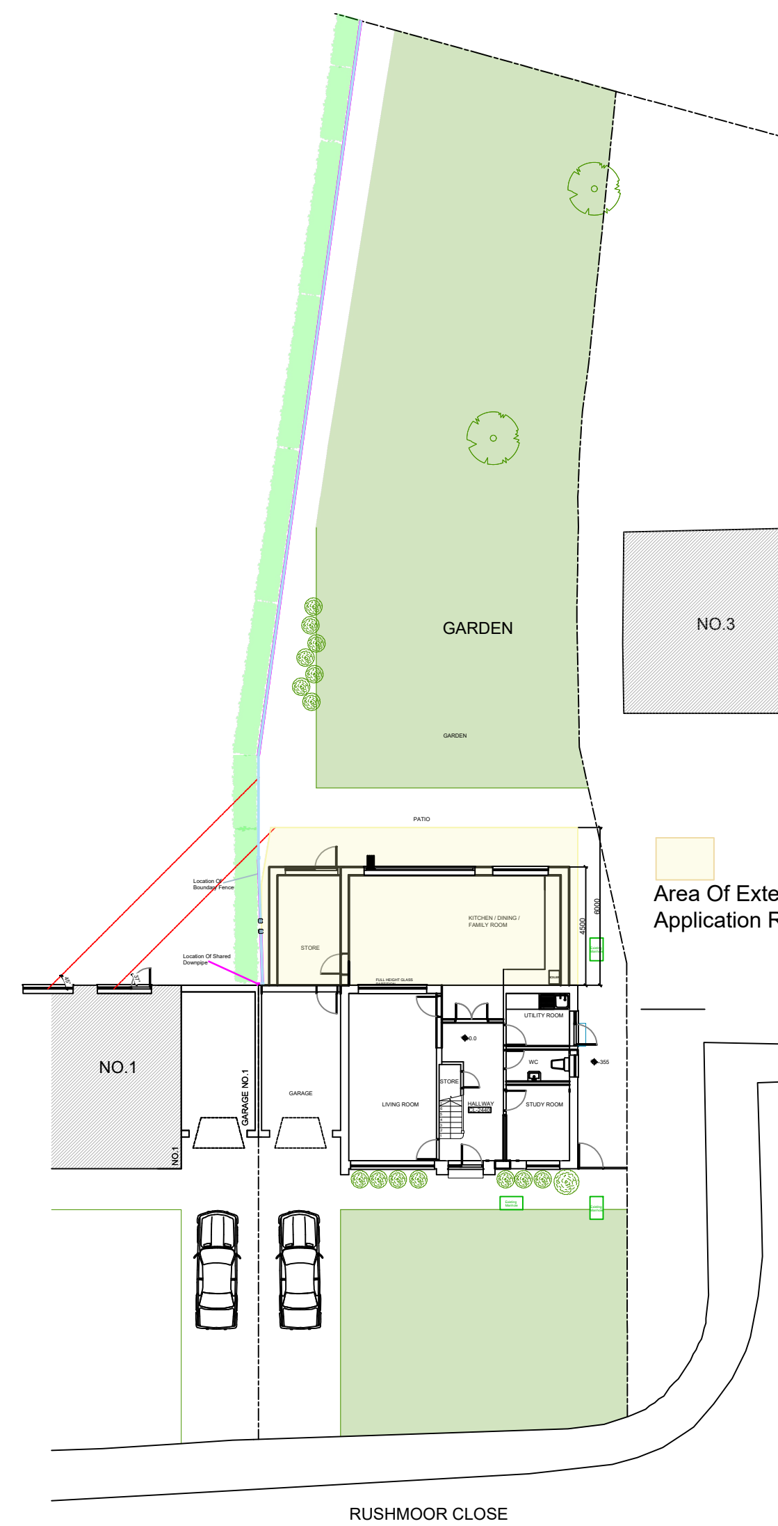
PROPOSED SITE PLAN 45 Degree Lines Shown From Neighbouring Ground Floor Windows SCALE 1:200
