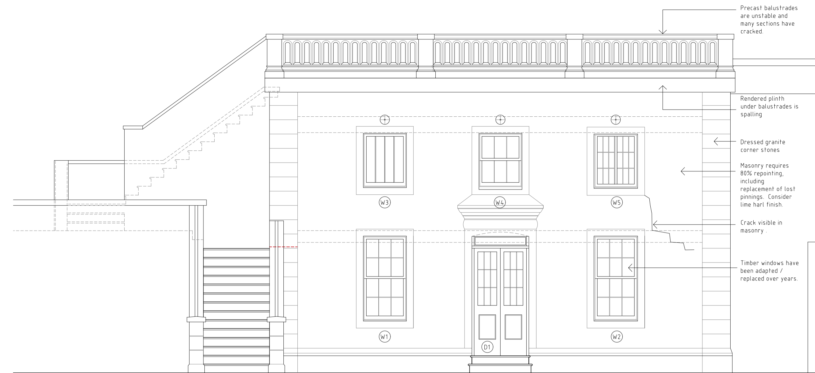
EXISTING SOUTH ELEVATION 1:50
