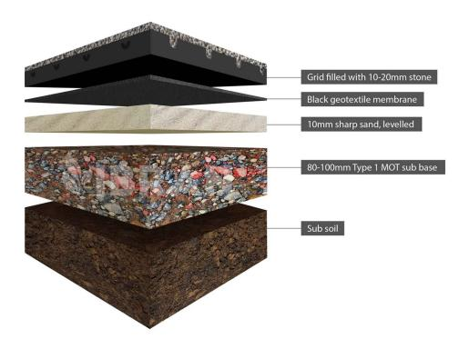
The grids are fully permeable, allowing uninterrupted flow of water from the top surface through into the sub base below, saving cost on additional drainage installation.
