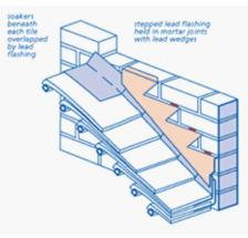
Where a pitched roof abuts the wall at an angle, a stepped cavity tray linked to a stepped flashing should be used. At roof abutments new joists to be supported on masonry walls with 47 x 150mm timber wall plate. Plate to be fixed to masonry with M10 resin anchors or thunderbolts at 450mm centres
