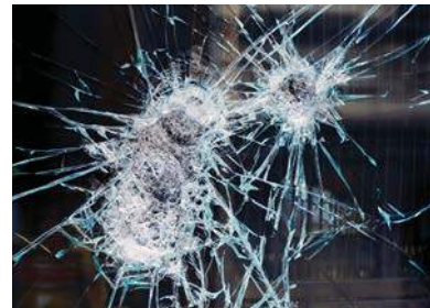
Laminated glass, retains the overall integrity of the glass.
