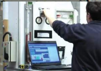
'Laboratory' tests for water ingress, wind resistance and air permeability
