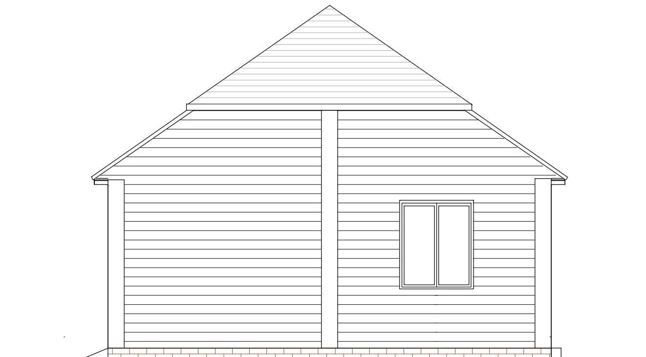
PROPOSED 35° ROOF PITCH SOUTH EAST ELEVATION
