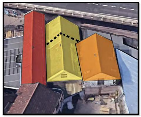
• The small flat roof section at the front of structure 2 will be demolished using a demolition rig, carefully separating the ties from the retained structure in the below photo:
