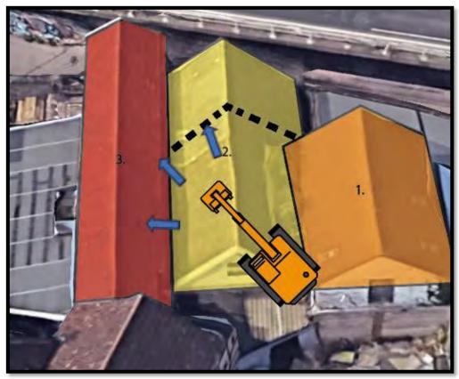
• The final sections of the third structure are to be demolished using the demolition rig, ensuring the fabric of the building falls internally within the footprint of the building
