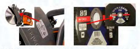
The speed marked on the wheel (disc) shown above must not be less than the max rpm of the machine. It can be the same rpm or a greater rpm.
