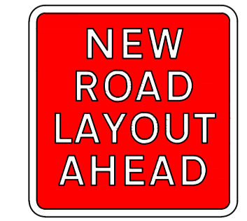
ROAD SIGN DIAG 7014 NEW ROAD LAYOUT AHEAD SIGN TO BE TEMPORARILY MOUNTED TO LIGHTING COLUMN IN VERGE MIN. 45m TO MAX. 150m AHEAD OF PROPOSED ROUNDABOUT SIGN TO BE REMOVED AFTER A PERIOD OF THREE MONTHS. REMOVAL DATE TO BE PRINTED ON REVERSE.
