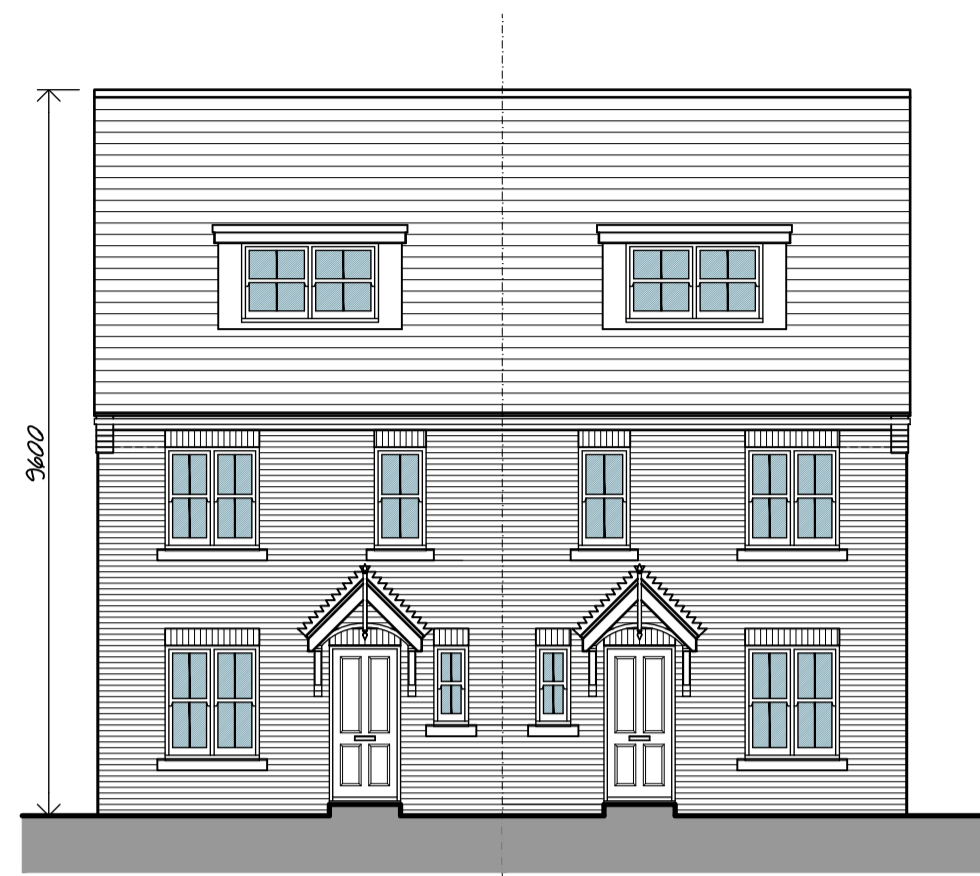
FRONT ELEVATION - BRICK
