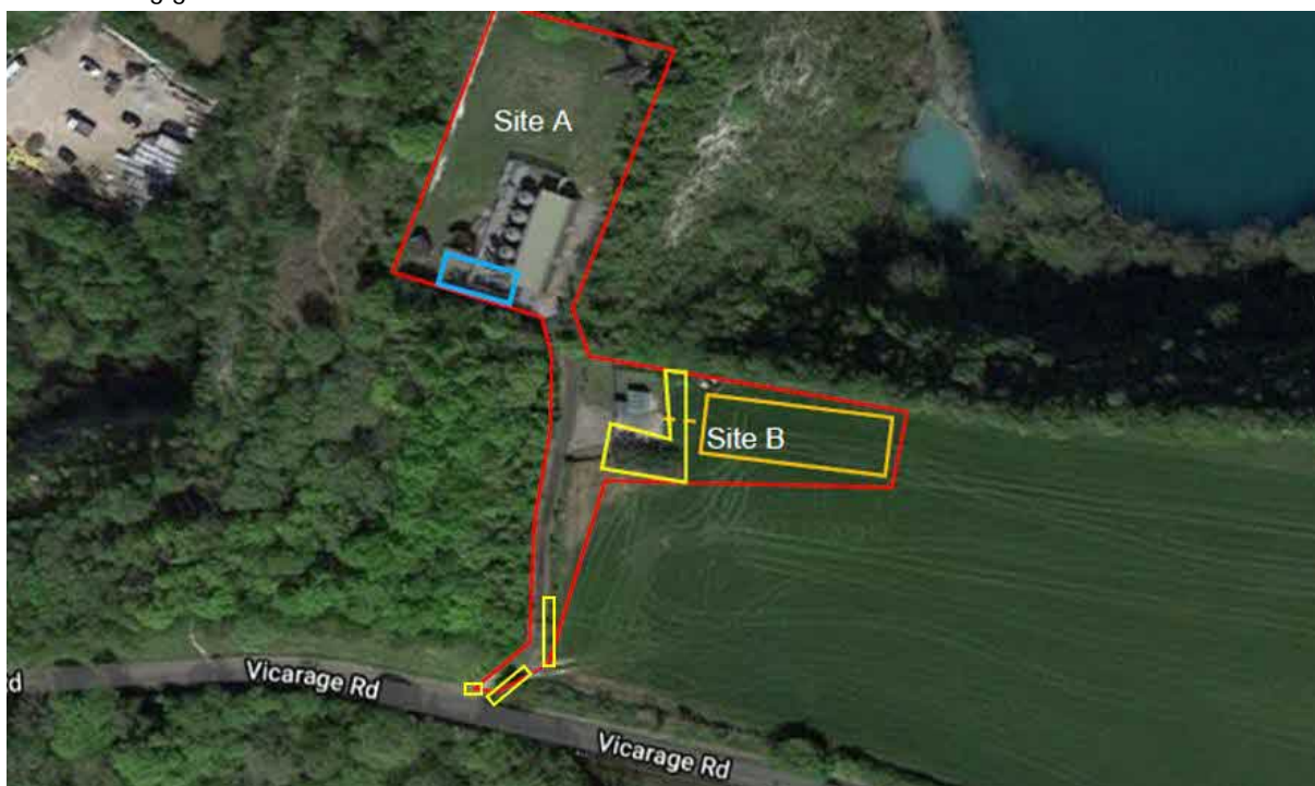
Figure 1: Location of Halling Greensand WTW, Kent. The orange outline is the indicative location of the new UV kiosk and access track, the blue outlines the proposed compound location within the WTW site, and the yellow area outlines the area of scrub/hedge to be removed to facilitate access to the works.
