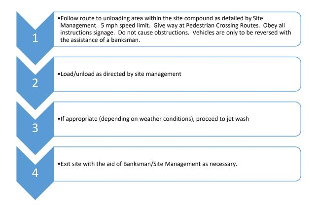
Site compound and storage is accessed via the main site access off Duck Street. Signage will be provided to safely and efficiently direct construction traffic and visitors off the existing highway and towards the Denbury Homes site compound and onsite parking facilities.
