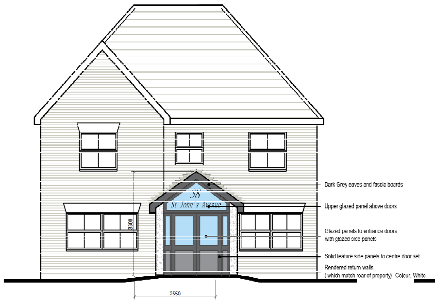
Existing Front Elevation (as built)
