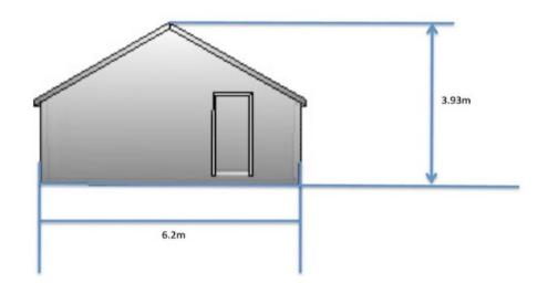
The garage will be constructed as a timber frame on a dwarf wall in brick, then clad in oak weatherboard. The roof will be in reclaimed tile to match the house roof. The finish and appearance will be similar to the detached garage in existence at our neighbours at Long Barn House.
