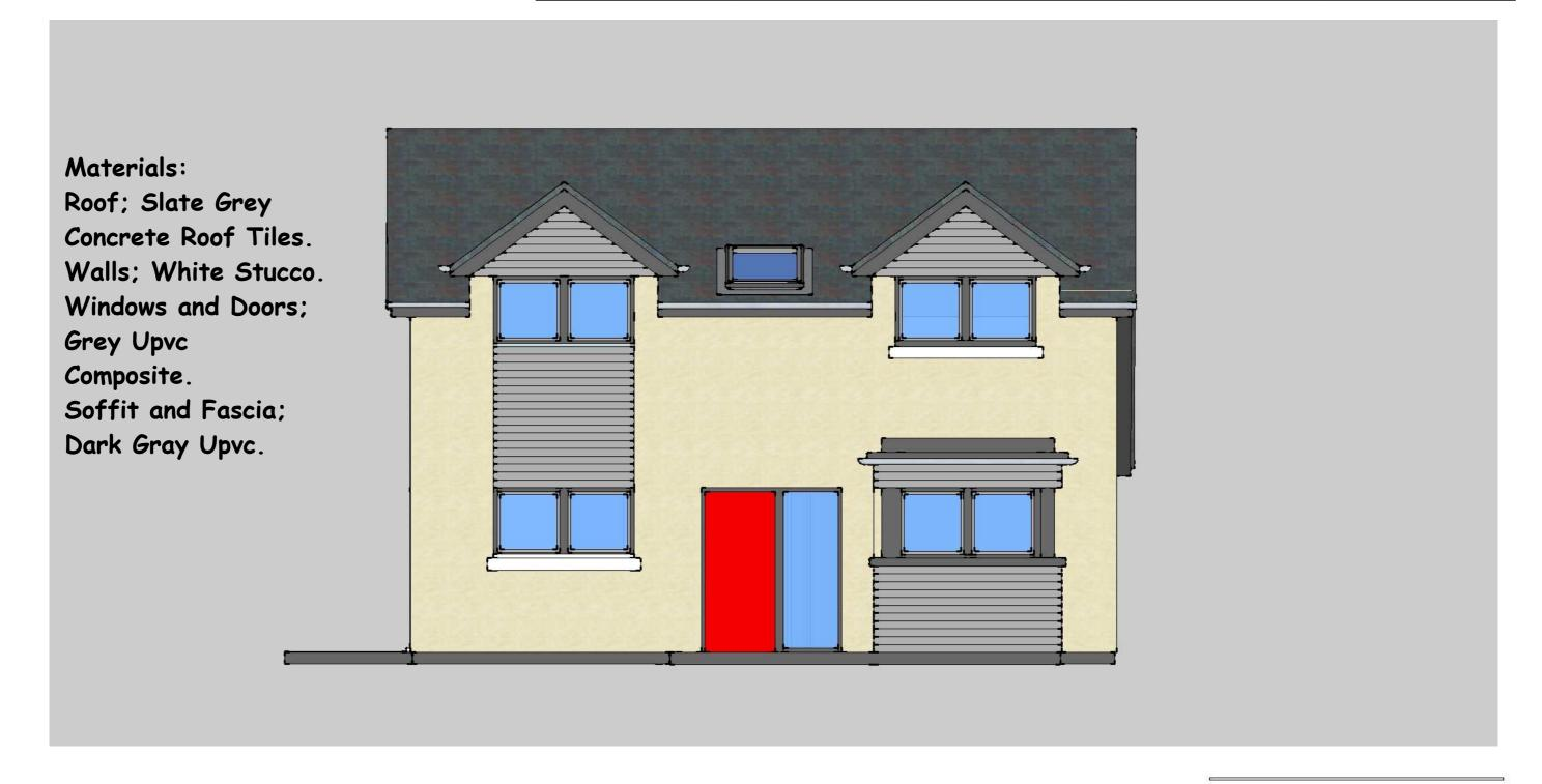
Muirhead Garage, 6 Newtyle Road, DD2 5PQ. 680\_05B, South Elevation, Unit 1. (basic).
