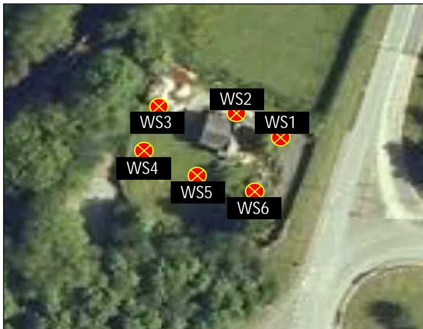
Figure 2: Borehole Location Plan
