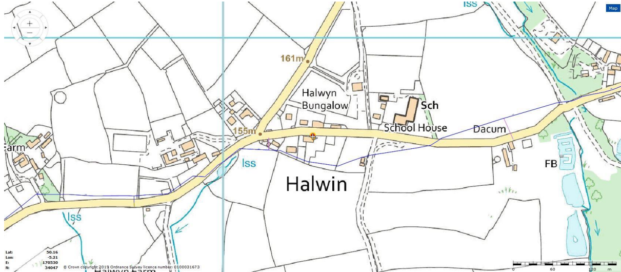
Fig 1. Extract of South West Water mapping showing that there are no sewers in proximity to the house
