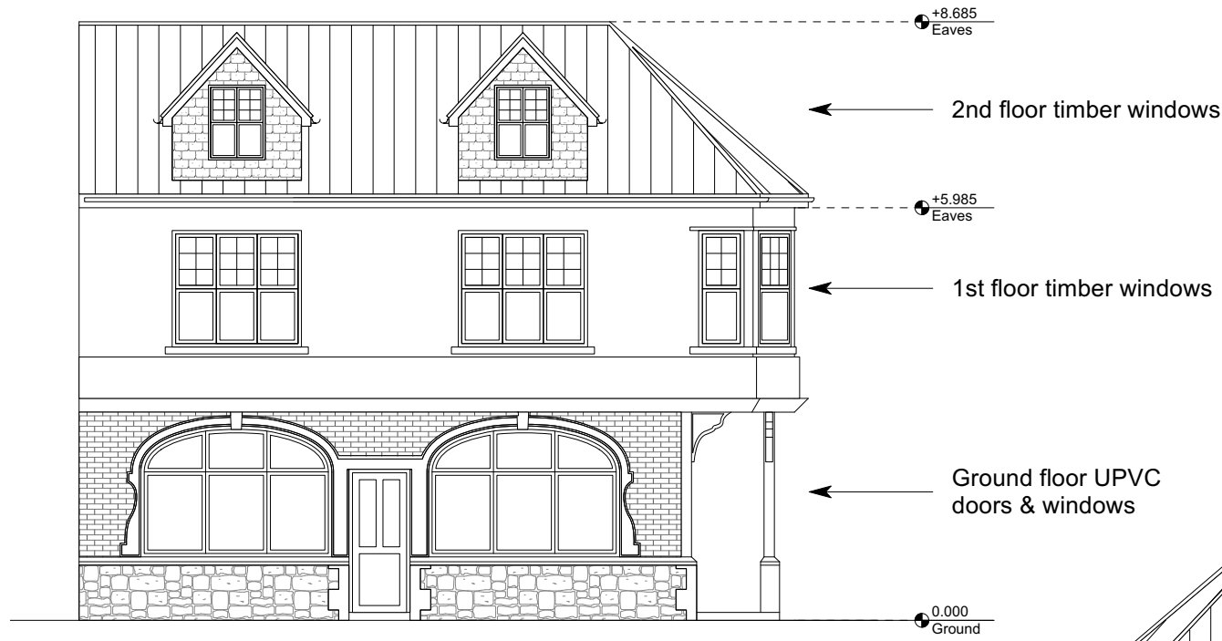
Front Elevation South West
