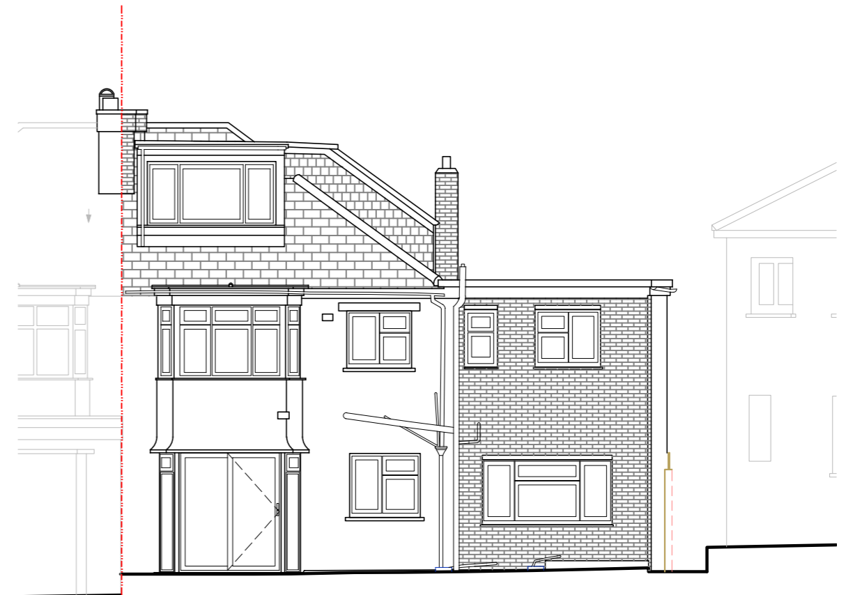
Figure 1 - Existing Rear Elevation - NTS
