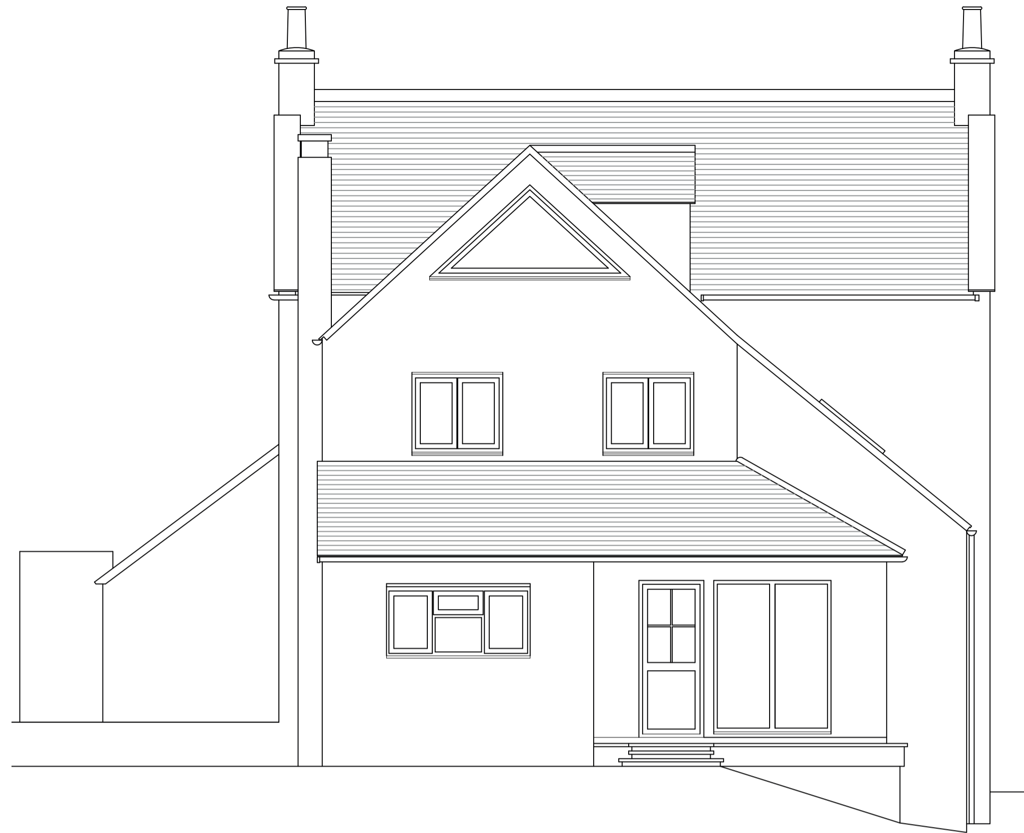
EXISTING REAR ELEVATION 1:50
