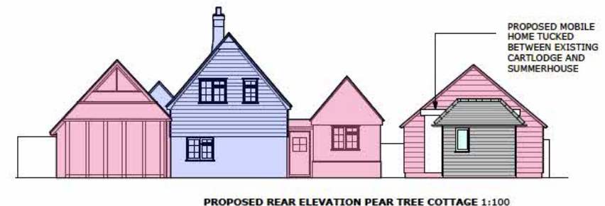
BLUE SHADING = ORIGINAL VOLUME OF PEAR TREE COTTAGE AS DESCRIBED IN LISTING DETAILS. PINK SHADING - LATER CONSTRUCTED ADDITIONS.
