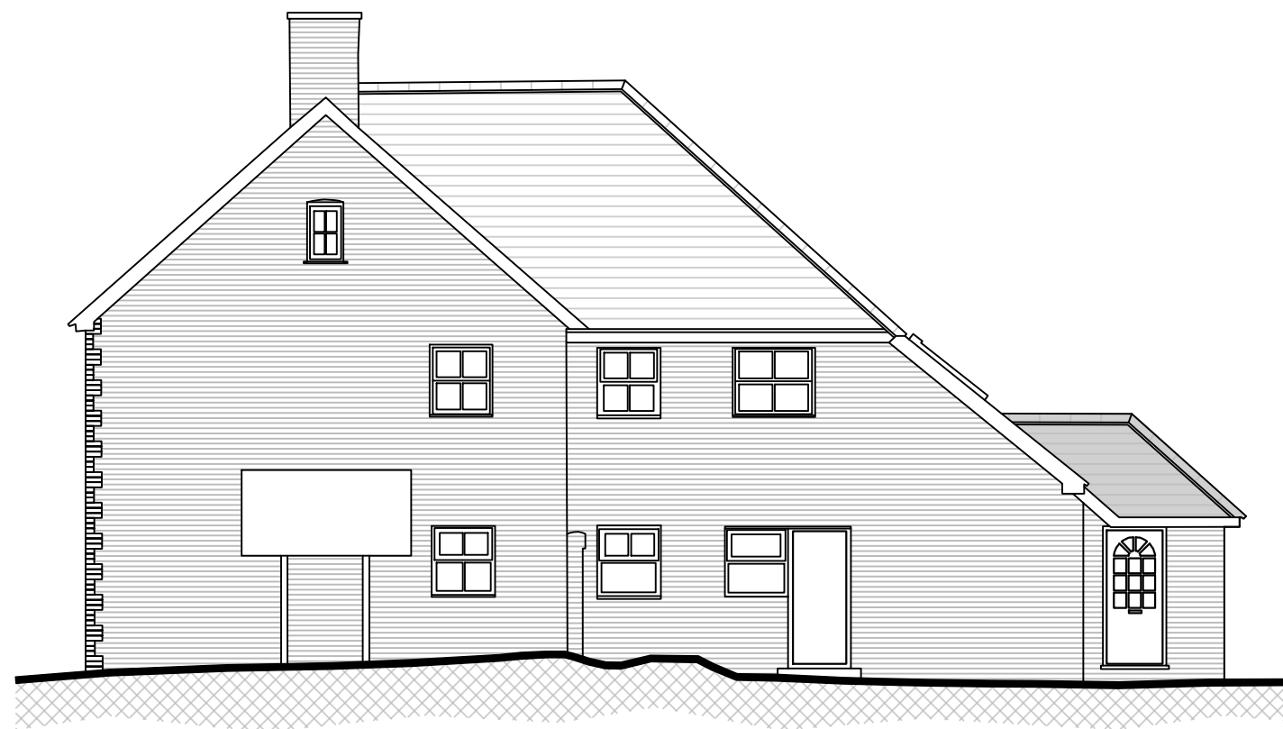
EXISTING NORTH ELEVATION SCALE 1:100
