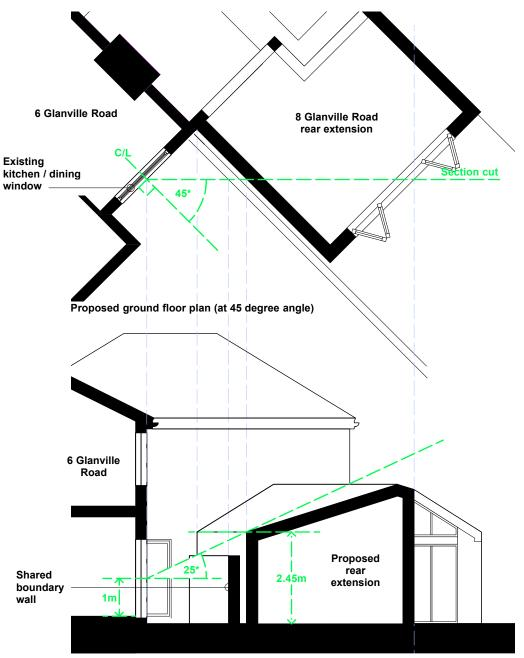
Proposed section (cut at 45 degree angle)
